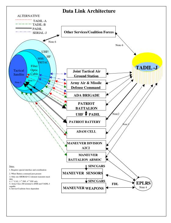
Figure III-2. Army Air and Missile Defense Data Architecture
